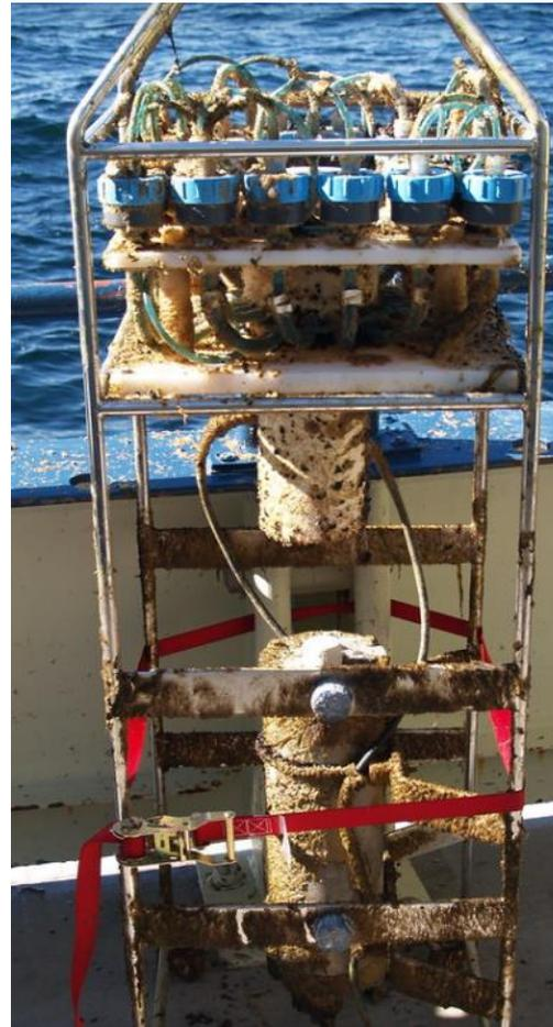
**Figure 3.** Example of biofouling of a Mclane Phytoplankton Sampler (photo from [www.mclane.com](http://www.mclane.com)).
