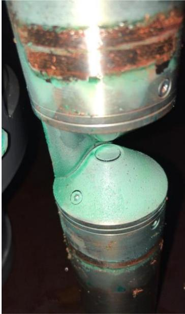
**Figure 4.** Example of copper precipitations from Cu on optical window. The sensor was enveloped by a copper net to avoid biofouling on the optical window. It turned out that the optical window was blinded by the Cu precipitations.
