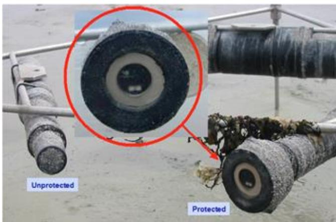
**Figure 5.** Biofouling protection by seawater electrolysis on turbidimeter Mont St Michel Bay – March to May – 80 days. On the left side, the unprotected turbidimeter shows significant coverage of barnacles after deployment. The protected turbidimeter, that uses a flat washer as a working electrode shows a clean transducing interface after the same deployment. Photo: Ifremer - L. Delauney.
